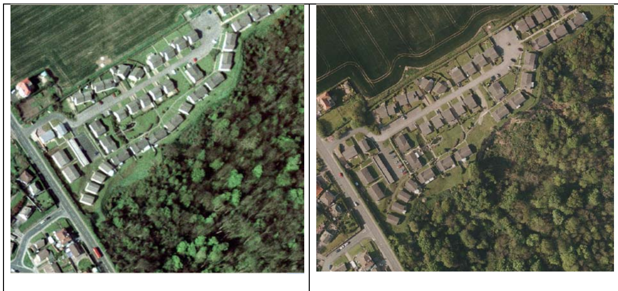
Figure 1. Qualitative comparison of vertical imagery from 1999 and 2010, highlighting landslide reactivation at Cayton Bay.
